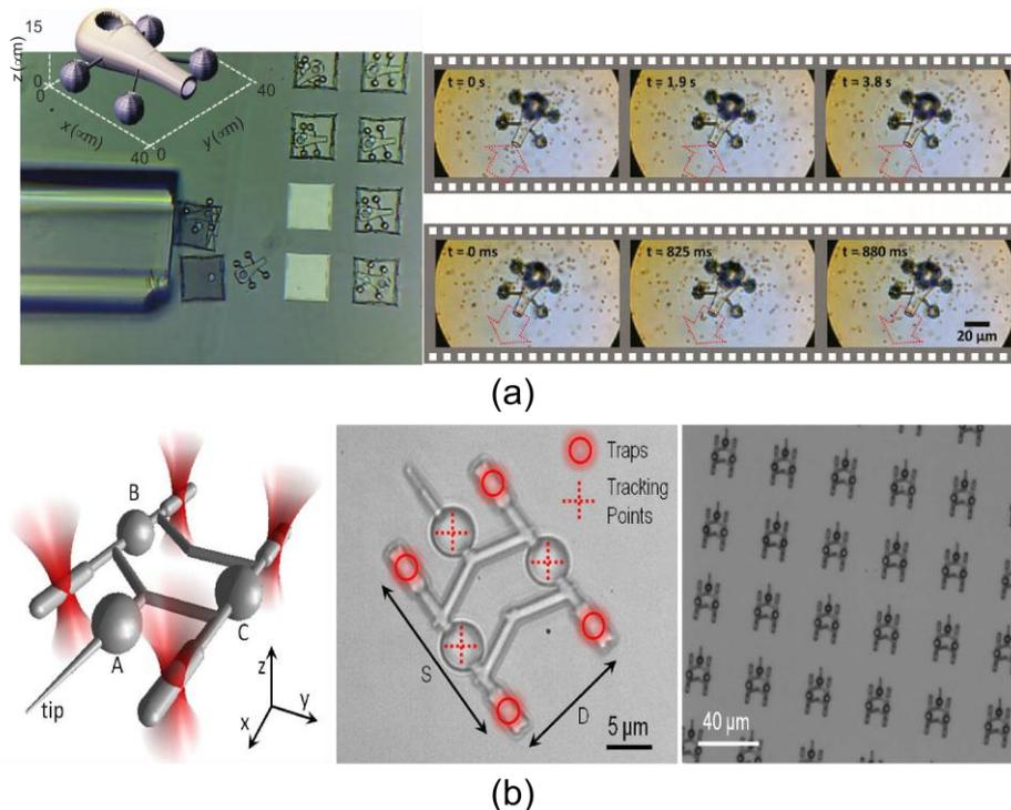
Figure 1: Examples of optical micro-tools. (a): Micro-tools for material transport via enhanced light-induced thermal convection. By changing the location of the beam in the metal layer, the micro-tool can be used to collect or eject the captured particles [6]. (b): Optical micro-tool design with four cylindrical trapping handles and three tracking points [8].
