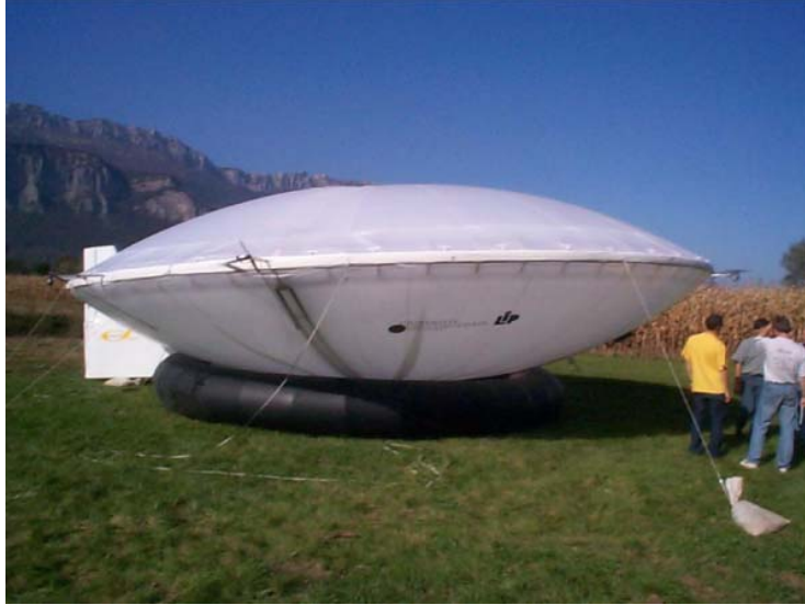
Fig. 1. A 10-meters wide lenticular blimp.
