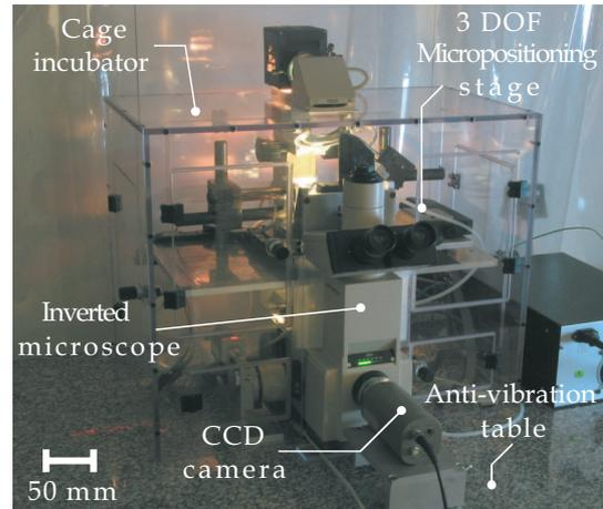
Fig. 1. The *FBM* experimental setup overview.
