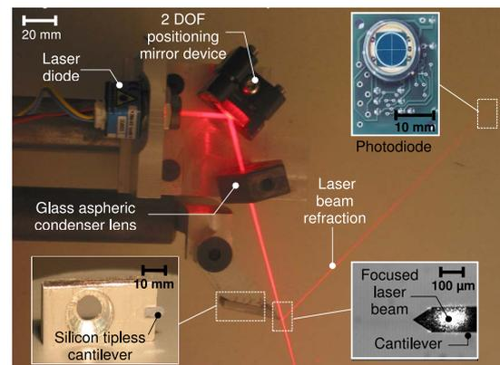
Fig. 2. The mechanical sensing unit.
