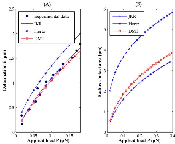
Fig. 11. (A) Estimation of the biological sample deformation  $\delta$  as function of the simulated load force  $P$  using Hertz, JKR and DMT theories compared to the experimental data. (B) Estimation of the contact area radius  $a$  using the Hertz, JKR and DMT theories.
