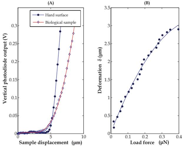
Fig. 6. (A) Experimental data of the photodiode output as function of the sample displacement performed on both single *EpH* cell and hard surface. (B) Experimental curve of the sample deformation  $\delta$  as function of the applied load by the cantilever.
