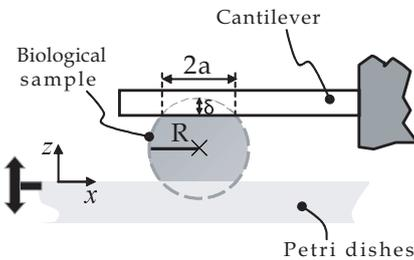
Fig. 10. Mechanical interaction scheme between the silicon tipless cantilever and the biological sample.
