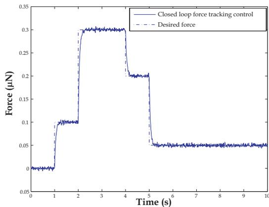
Fig. 3. The force feedback control approach.
