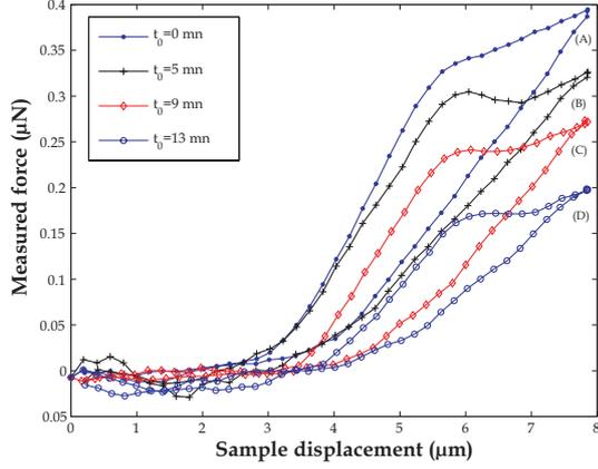
Fig. 9. Evolution of the measured force as function of the sample displacement for different elapsed times  $t_0 = 0, 5, 9$  and  $13$  mn.
