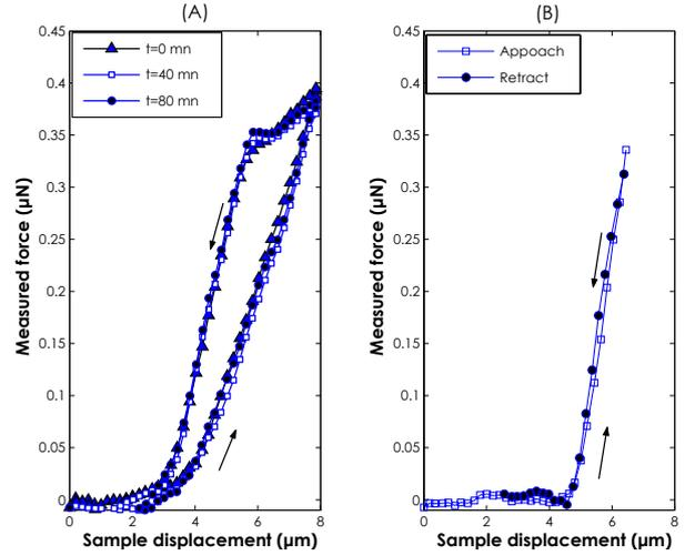
Fig. 7. (A) Experimental spectroscopy curves (approach and retract) performed on a single *EpH* cell at different time intervals ( $t=0\text{ mn}$ ,  $40\text{ mn}$  and  $80\text{ mn}$ ). (B) Single referenced approach and retract curves performed on hard surface.
