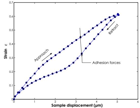
Fig. 8. Dimensionless strain per module length  $\varepsilon$  as function of the sample displacement  $\Delta z$ .
