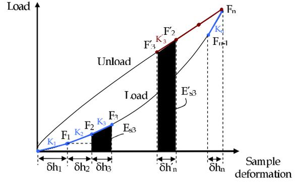
Fig. 3. A typical load-elongation diagram for soft tissue.
