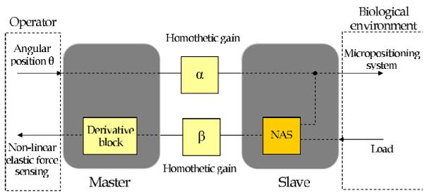
Fig. 4. Overview of the Master/Slave bilateral coupling scheme.
