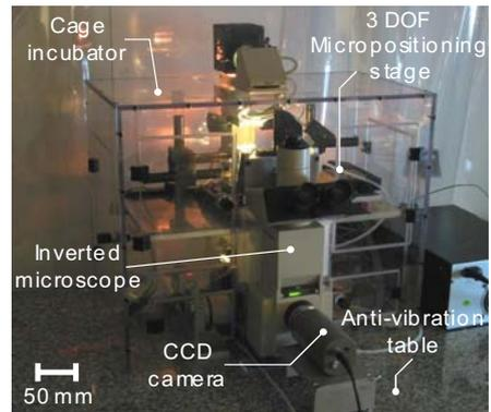
Fig. 1. The *FSBM* experimental setup overview.
