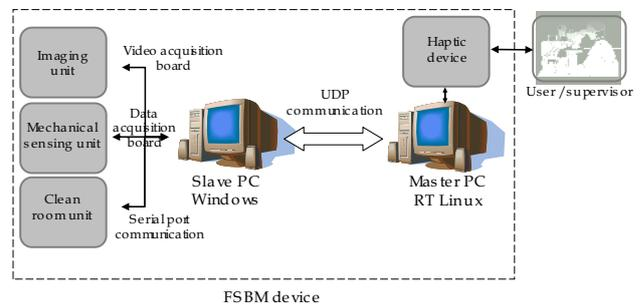
Fig. 2. Block diagram of the *FSBM* device.
