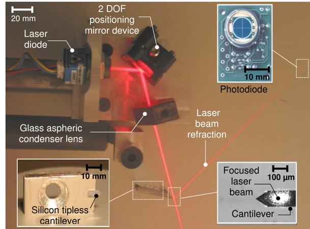
Fig. 2. The mechanical sensing unit.
