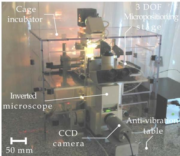
Fig. 1. The FSBM experimental setup overview.
