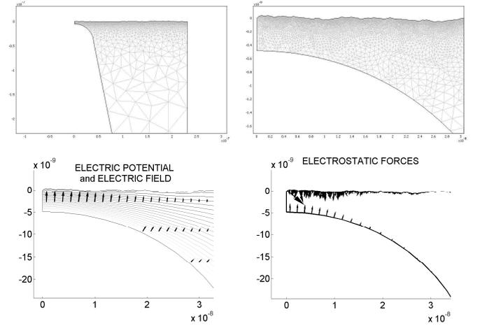
Fig. 5. Different representation of the geometries in contact (cone and plane) with a roughness for the plane simulated with  $D=1.55$ ,  $G=1.5 \times 10^{-12}$ ,  $\gamma=1.5$  and  $L=1\mu\text{m}$ .
