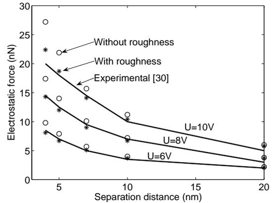
Fig. 6. Electrostatic normal force (nN) versus separation distance (nm) for different applied voltage for a sphere-ended conical tip of radius  $40\text{nm}$  and half aperture angle  $\theta=10^\circ$ . Plot shows experimental results obtained by Sacha et al. [30], simulations results without roughness parameters and simulation results including roughness parameters  $G = 1.5 \times 10^{-12}$  and  $D = 1.55$  chosen in order to get a maximum asperities height of the order of  $1\text{nm}$ .
