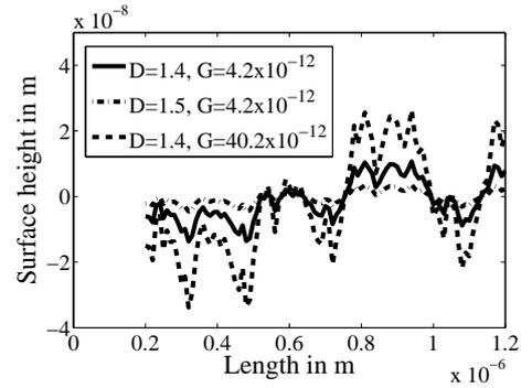
Fig. 2. Illustration of the influence of the fractal parameters  $D$  and  $G$  on the profile.
