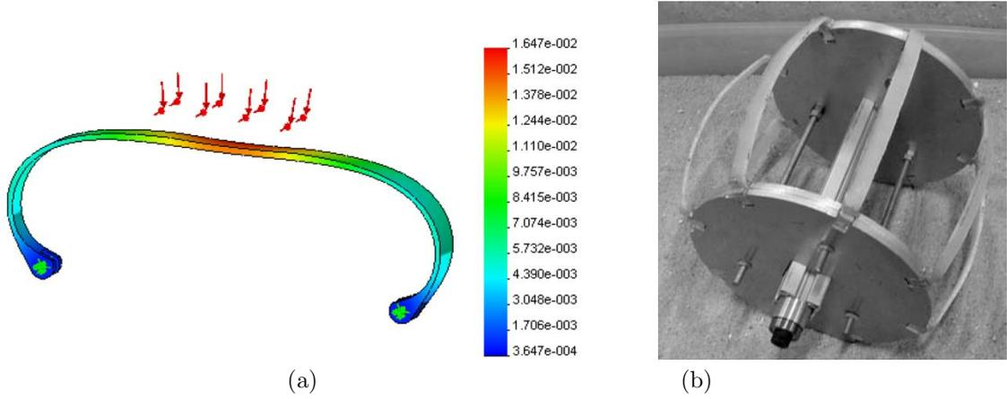
Fig. 9: (a) Elastic tread adaptation mechanisms with arc-shaped beam; (b) First prototype
