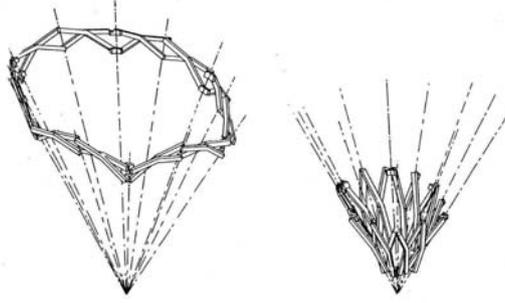
Fig. 3: Configuration where the pivot points of all the scissor-pair lie on a circle
