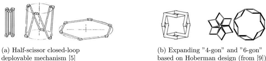
Fig. 2: Closed-loop deployable mechanisms
