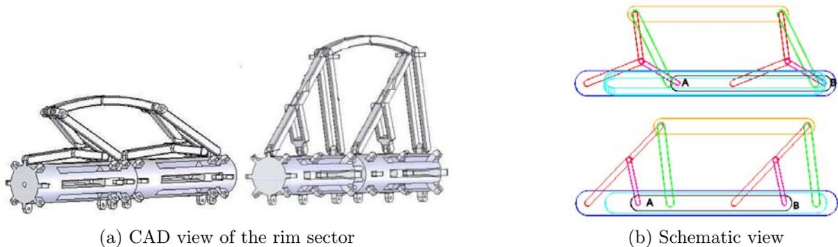
Fig. 4: Mechanism used for the expansion of the rim
