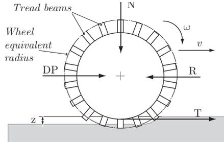
Fig. 10: Wheel ground interaction forces
