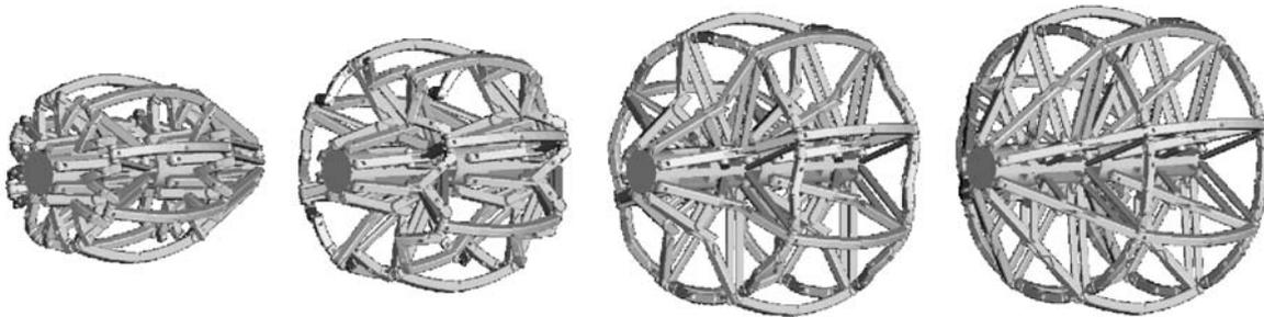
Fig. 6: Preliminary concept : folding/unfolding process.
