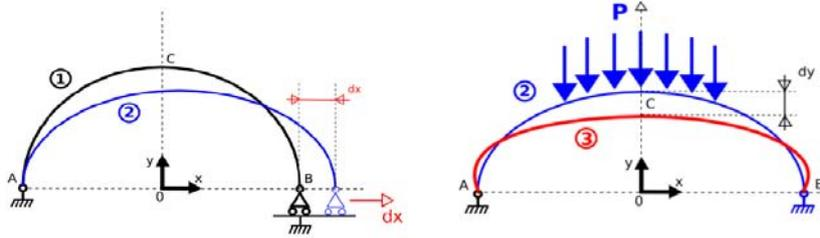
Fig. 11: Elastic deformation of a arc-shaped beam
