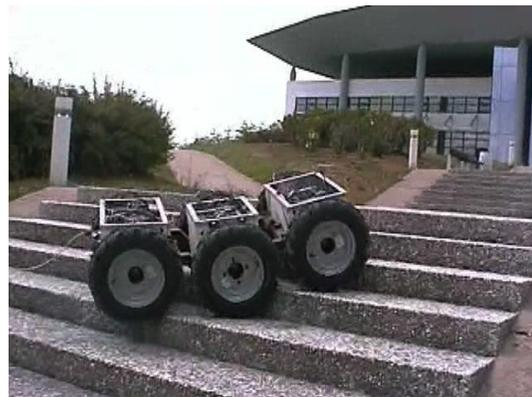
Fig. 1. The RobuRoc mobile robot climbing a stair
