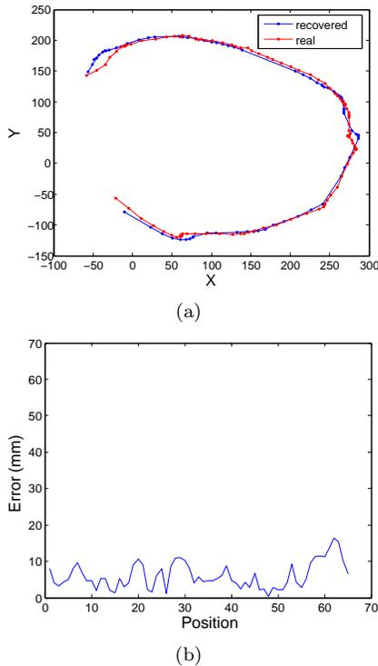
Fig. 10. (a) Trajectories computed from the correct shapes with the synchronization method (blue curve) and the segmentation method (red) in the plan  $XY$ . (b) For each position, the blue curve is compared to the red one by measuring a "point-to-point" error. The mean error (5mm) is reasonable small enough compared to the magnitude of the trajectory ( $\sim 35\text{cm}$ , the error is less than 2%).
