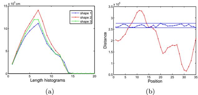
Fig. 9. (a) Characterization vectors for 3 reconstructions. The red one is the histogram of an exact reconstructed car i.e. the frames are synchronized. (b) Correct shapes (blue dots) can be extracted from available reconstructions since they have little dispersion around some mean value. Some geometrically correct shapes but not time complying are represented by red dots inside the blue area. These cases appear when their (exact) time shift is not far (but bigger) from the estimate one.
