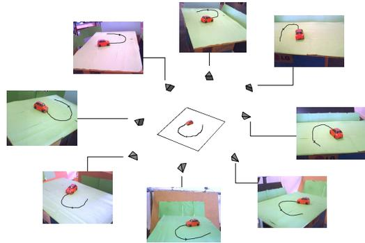
Fig. 8. Experimental system of 8 cameras observing a mobile vehicle that describes a planar trajectory. A camera seeing the scene from the above is used to segment the vehicle. Two markers are placed on it to ease the segmentation process. We can determine the position and the orientation of the car in each image of the sequence. The trajectory (black curves) of the car is computed and can be used as reference curve for comparison purpose.
