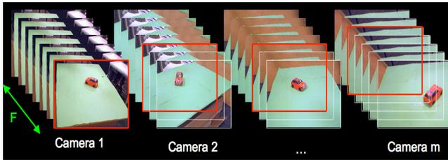
Fig. 7. For each frame of  $C_1$ , an interval of length  $f$  is set. This defines locally a set of images acquired by the  $m$  cameras, then reconstructions are performed by combining frames from each camera.
