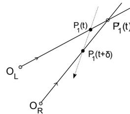
Fig. 4. Due to the delay, the point  $\mathbf{P}'_1$  is constructed from points  $\mathbf{P}_1(t)$  and  $\mathbf{P}_1(t + \delta)$  seen by  $C_L$  and  $C_R$ .
