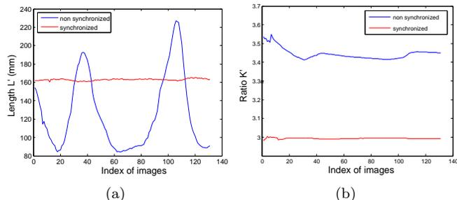
Fig. 6. (a) If the frames are synchronized, the computed lengths of reconstructed segments are stable around the mean value (red curve). On the other hand, if frames are unsynchronized, the dispersion is much more important (blue curve). (b) We observe the same result for the ratio  $K$ . Figures (c) and (d) present the corresponding errors.
