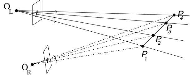
Fig. 2. If the images from the cameras  $C_R$  and  $C_L$  are synchronized, the points  $\mathbf{P}_1, \mathbf{P}_2, \mathbf{P}_3$  and  $\mathbf{P}_4$  can be correctly reconstructed from images.
