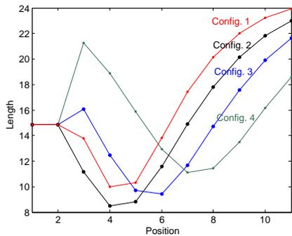
Fig. 5. Computed lengths of  $\mathbf{P}_1\mathbf{P}_4$  for several arbitrary fixed  $D'$ . The initial length  $D$  is set to 28 cm. For readability purpose, only some curves are presented and we can see that the estimate length in each case is not constant.
