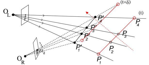
Fig. 3. The cameras  $C_R$  and  $C_L$  are unsynchronized. The projection from image to space produces the shape  $\mathbf{P}'_1\mathbf{P}'_2\mathbf{P}'_3\mathbf{P}'_4$  at different positions according to the rigid body hypothesis.
