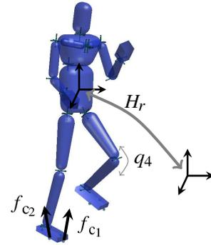
**Fig. 2** The virtual human with 36 active dof and the homogeneous transformation matrix accounting for the position of the free floating reference body (the pelvis).
