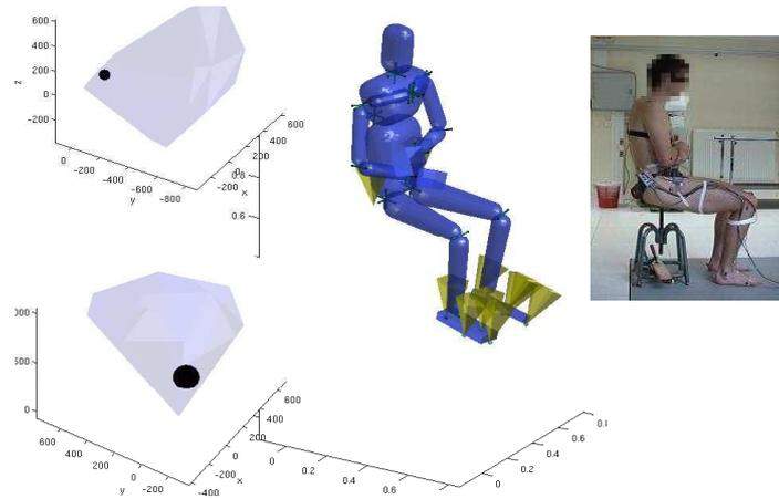
**Fig. 3** (right) The virtual human at the beginning of the sit-to-stand motion, in contact with the ground and the seat. The linearized friction cones appear in yellow. (top left) Resistable contact moment (numerical values in Nm). (bottom left) Resistable contact force (numerical values in N).
