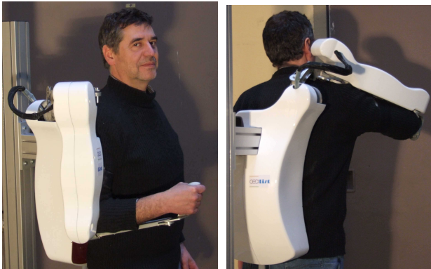
Fig 1. ABLE 4 axis exoskeleton actuated by screw-and-cable actuators
