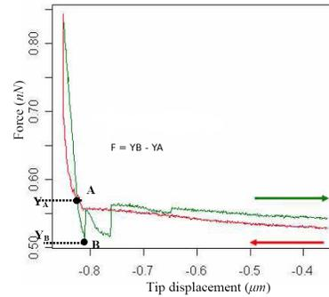
Fig. 1. Force (nN)/distance ( $\mu m$ ) curve.  $F$  is the breaking force value. (red) approach step, (green) retreat step. Several discrete steps appear. We suppose that the most probable reason is the hydrogen bonds breaking and the reorganization of the molecule or ultimately DNA breaking.
