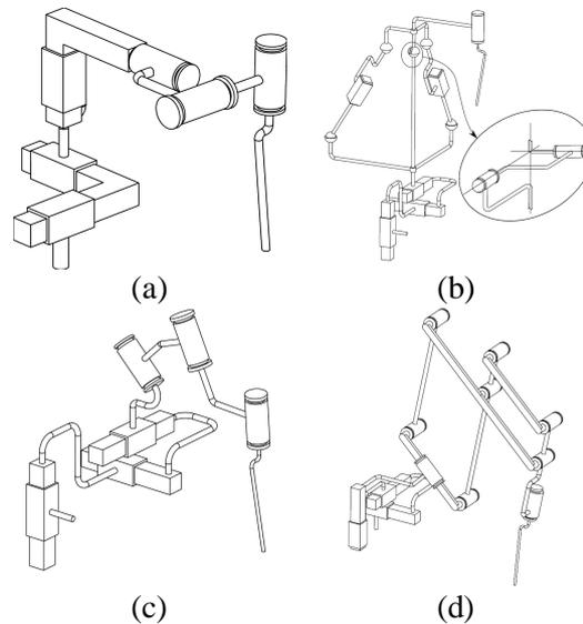
*Fig. 3: Kinematic candidates: (a) 6 dof series, (b) 6 dof mixed, (c) 6 dof series with offset rotation centre (orc), (d) 6 dof Evans with orc*
