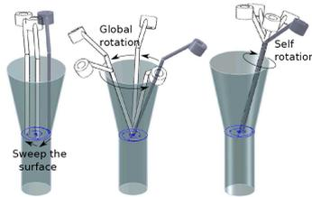
Fig. 6: Tool representative trajectory used for the optimization process
