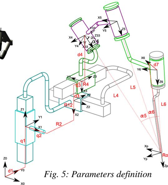
Fig. 5: Parameters definition
