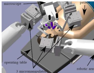
*Fig. 1: Overview of a possible assistance robot for the middle ear surgical intervention*
