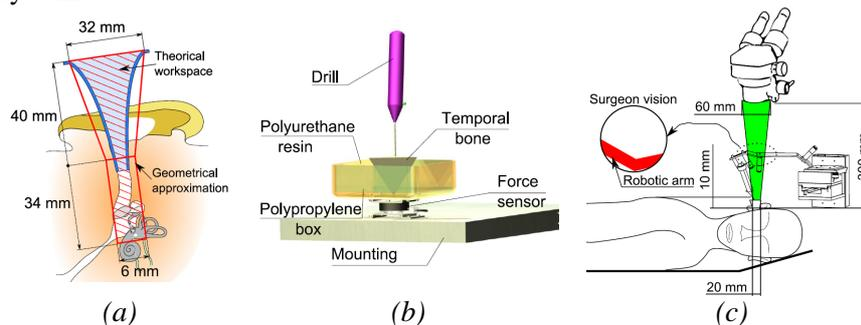
Fig. 2: From left to right, (a) geometrical approximation of the workspace, (b) experimental setup for measuring the forces, and (c) a global view of the intervention environment
