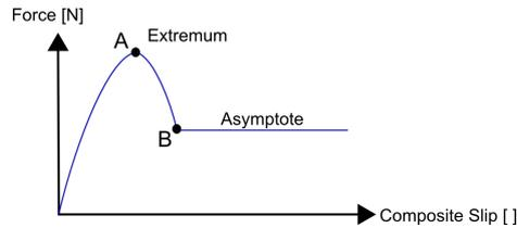
**Figure 3.** Friction Model
