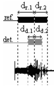
Fig. 4. Sensitivity to the duration from the detected vowel segments (black) according to the reference ones (gray)
