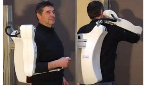
Fig. 7. ABLE 4 axis exoskeleton actuated by screw-and-cable actuators
