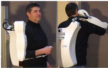
Fig. 5. ABLE 4 axis exoskeleton actuated by screw-and-cable actuators
