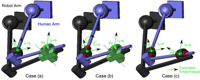
Fig. 8. Schematic of possibilities for coupling ABLE to an human arm. Case (a): ball joint alone at  $P_1$  and ball joint on 2 slides at  $P_2$ ; case (b): Universal joint + 1 slide (in red) at  $P_1$  and ball joint on 2 slides at  $P_2$ ; case (c) Ball joints with slides (in red) at both  $P_1$  and  $P_2$ .
