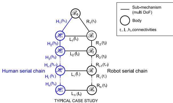
Fig. 1. Schematic of two serial chains parallel coupling
