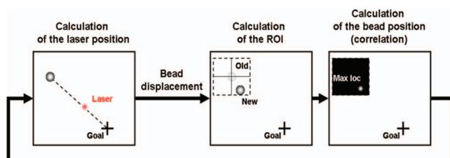
FIG. 4. Schematics of the tracking method using image correlation. The laser is shot at a distance  $d$  from the bead to handle it, the bead moves towards the laser beam and then the ROI image updates its position in order to not to lose the future bead position. Once the bead position computed, the laser is shot again at the same distance  $d$ . This continues until beads reach their target positions.
