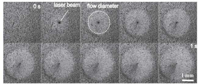
FIG. 2. Diameter of the convection cell depicted by pictures captured every 10 ms (100 Hz with  $500 \times 500$  pixels per image). Images are shown every 110 ms. Hollow glass beads of 8 up to  $12 \mu\text{m}$  in diameter, which density is similar to water, were used as tracers in a depth of water of  $150 \mu\text{m}$ .
