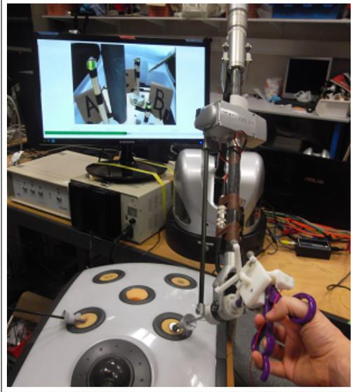
Fig. 1. Subject point of view for laparoscopic surgery task with kinaesthetic and visual feedback. On the bottom right, the subject's hand manipulates the laparoscopic tool fitted with optical tracking markers. A haptic interface is also attached to the shaft of the tool just below the handle and acts as a co-manipulator. The subject is presented the view from the endoscope on the screen seen at the top left of the image.
