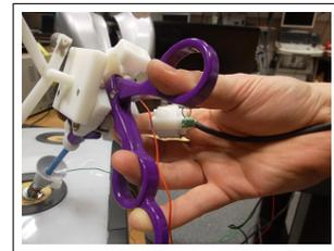
Fig. 3. ERM vibrating motor attached to the subject's hand
