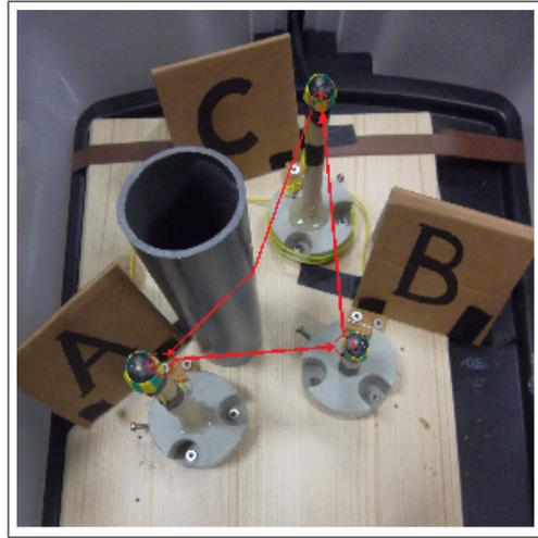
Fig. 2. View from above the inside of the laparoscopic training simulator. The red circles highlight the electrical contacts on each of the three pegs and the arrows show an example of trajectory to be followed. An obstacle is placed on the [AC] trajectory in order to further complicate the task and assess the impact of the provided feedback when trajectories became less intuitive.
