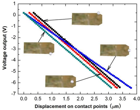
FIG. 2. (Color online) Examples of the sensitivity calibration on four different contact points (see four corresponding scaled images) on the cantilever. In which three curves with the same gradient present the contact points on the hemline of the trapezoid head on the free end of the cantilever. The fourth curve with a lower gradient denotes the calibration result when the contact point is on the tip of cantilever.
