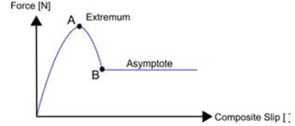
Fig. 6. Friction model
