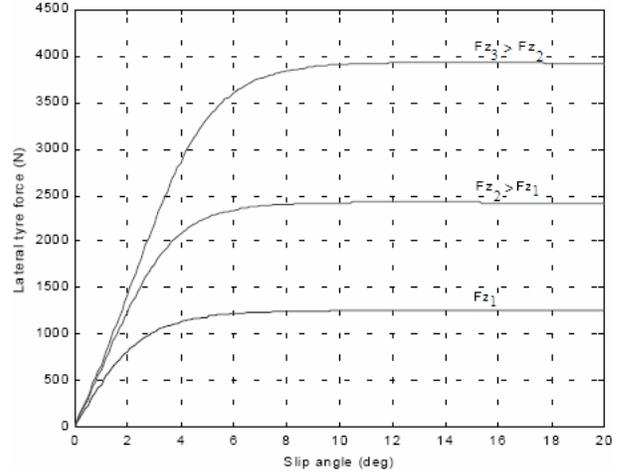
Fig. 3. Empirical model of lateral force vs slip angle (adapted from [9])
