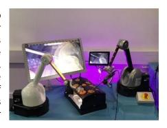
**Objectives:** With this project, we propose to study the contribution of augmented reality in the operating room. Its specificity project is to take advantage of the possible complementarity between comanipulator robotic arms held by the surgeon and an augmented reality device carried by the latter (Hololens/Varjo XR1).
